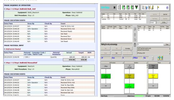
Integrated weighing equipment to achieve integrated material weighing management: by scanning the material label to determine the correctness of the material, automatically calculate the material demand, obtain weighing data, print weighing label, generate weighing report, ensure that the weighing process meets the production requirements. The system supports net weight
